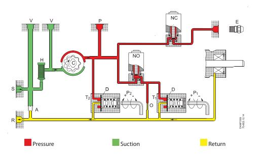
From the suction inlet (S) oil is drawn through the filter (H) to the gear set, where the pressure is increased. By means of the diaphragm (D) in the pressure regulator for stage 1 (T1), the pressure is kept constant at the value set on adjustment screw (P1).
