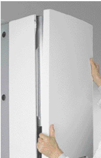
Removal of the casing front and side panel by vertical sliding
