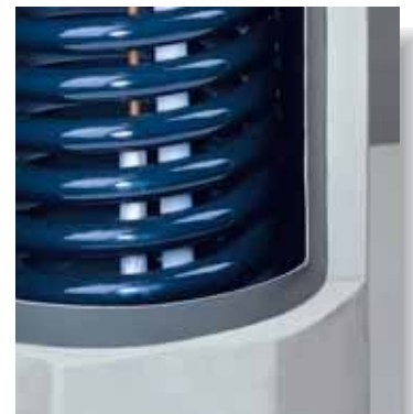
150 litre capacity, electronic de-stratification system, rapid storage cylinder, enamelled according to the standard DIN 4753, complete with magnesium anode and insulated in high density polyurethane.
